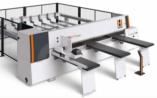
The integrated linear guide concept is the unbeatable highlight. For example, the sawing carriage moves completely on linear guides inside the machine. This provides absolute production reliability, speed and performance. The new TECTRA series is also way ahead of the game when it comes to safety. The DGUV\* certification means it meets the highest safety standards – your guarantee of a safe workplace.
